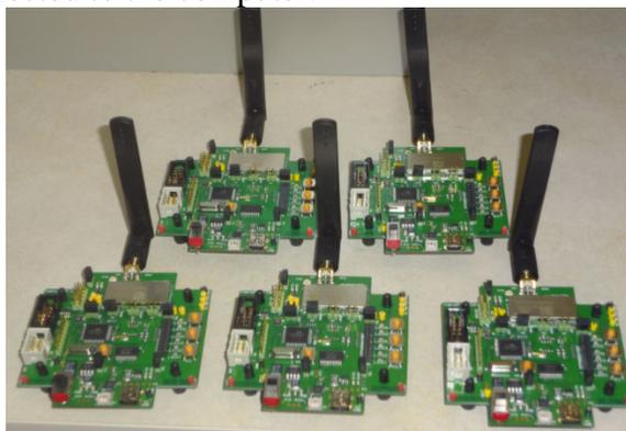
Figure 1. Nanotron swarm nodes (swarm of 5 nodes)
