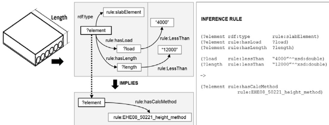
**Figure 4** Basic example of a rule (in JenaRule language) allowing to infer the most appropriate calculation method (namely, rule:EHE08\_50221\_height\_method) for elements of type rule:slabElement with a load less than 4000 KN/m<sup>2</sup> and a length less than 12000 millimetres.
