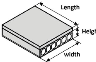
The diagram shows a 3D perspective of a hollow-core slab. It is a rectangular block with several circular voids along its length. Dimension lines indicate 'Length' along the top edge, 'Width' along the bottom edge, and 'Height' along the right side edge.
