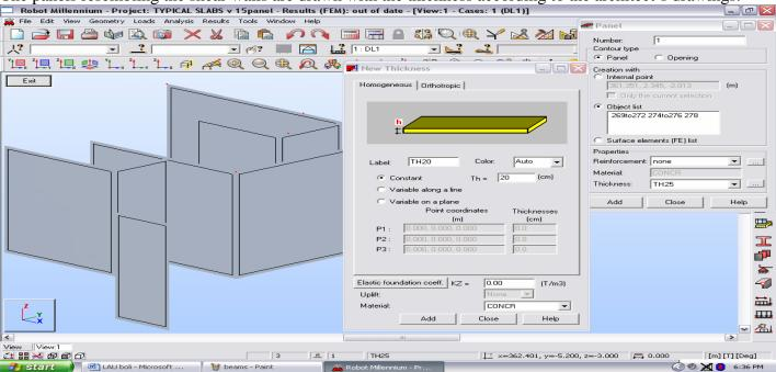
The slab contour is drawn with a thickness and the orthotropic slab system is used to define the joist slab.
