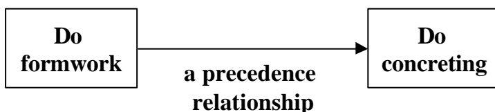
Figure 6. An arrow between two tasks indicates a precedence relationship.
