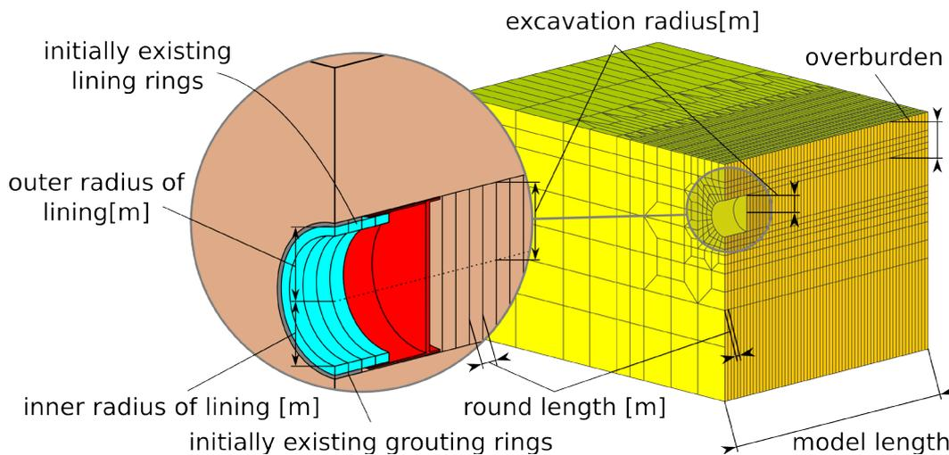
Fig. 4: Geometrical parameters of the FE simulation model.
