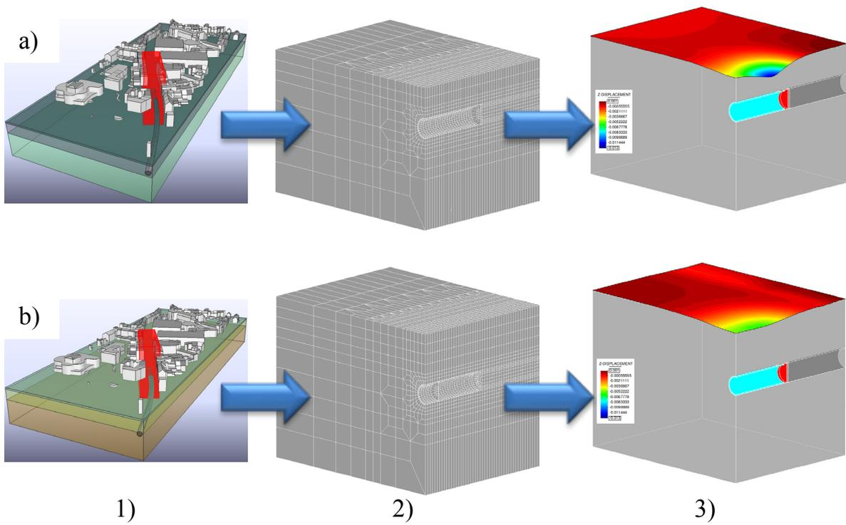
Fig. 6: Workflow (steps 1 to 3) of model mapping for an overburden of 1.5D (a) and 2.5D (b).
