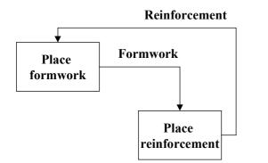
Fig. 4. The modelling of feedback in IDEF0.
