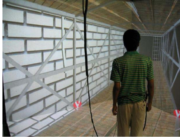
Figure 5: A virtual scaffolding observed by a real user. There is a virtual wire hanging on the wall to the left of the black, real cable used to control the immersive display. The display consists of three screens below visible to the user's left and right.
