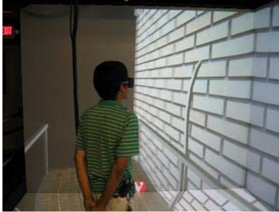
Figure 1: A virtual scaffolding observed by a real user on the top level of the building. There is a virtual wire hanging on the wall.
