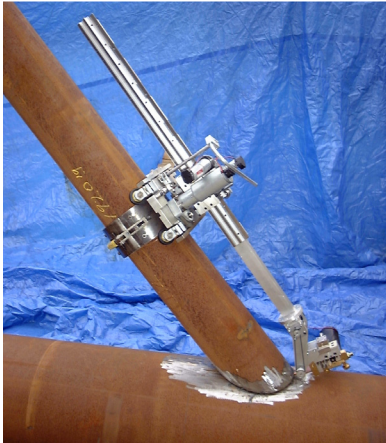
Figure 9. Prototype welding hardware for tubular nodes
