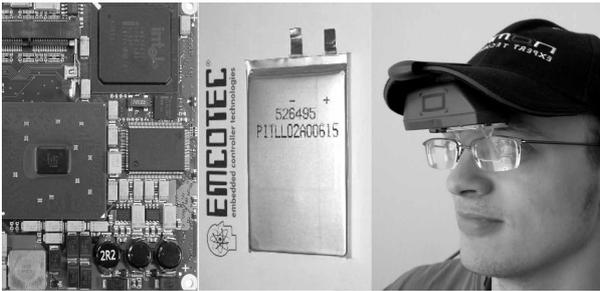
Figure 15: Using commercially available components, Left: PC-mainboard (3.7x4.5" , Pentium® M 1.6 GHz, 512 MB), Middle: Rechargeable batteries from model building technology, Right: Retinal display system [15]
