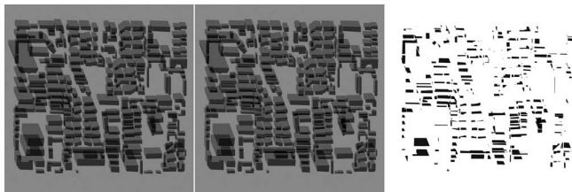
Figure 4: a) top view of Yanzi-Shan with transparent buildings at 10:30 December 21; b) marked areas are the dark shadows, c) the map of dark shadows (projection of shadows casted on buildings' surfaces) generated in Adobe Photoshop.
