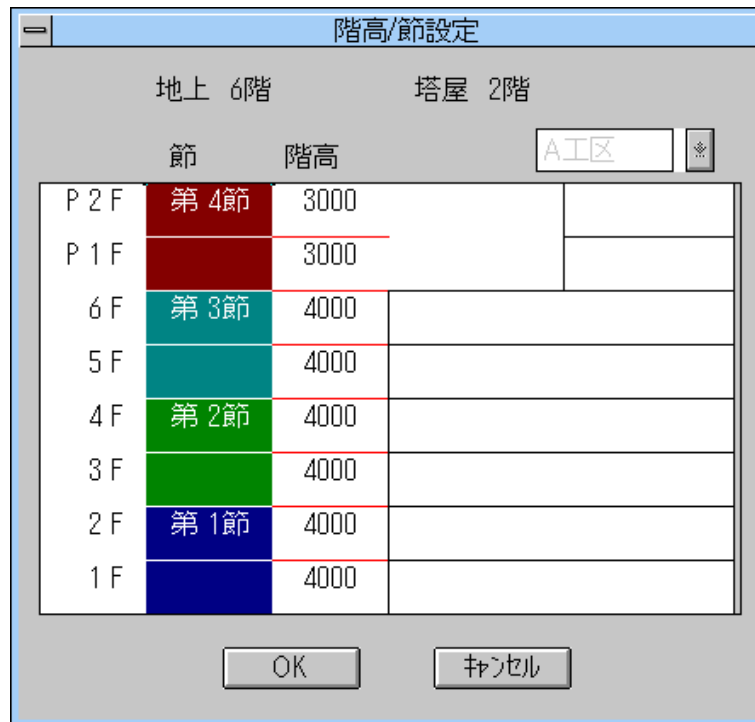
Figure - 4: Definition of Floor and Erection Stage
