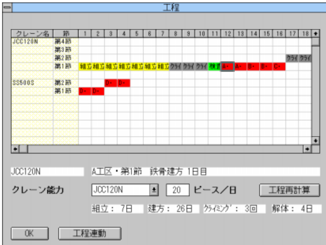
Figure - 6: Lifting and Climbing Schedule Evaluation
