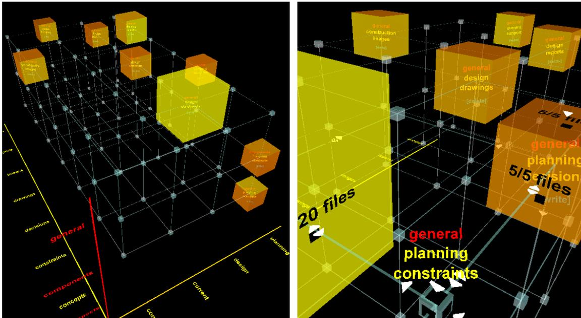
Figure 4. A 3-dimensional visualization of the organizational structure of a project. Component cubes are sized with respect to document count, and highlighted in the structure according to selected criteria, e.g., whether there are new documents or documents waiting attention. Each cube links to an overview of the relevant documents. Bige Tunçer.
