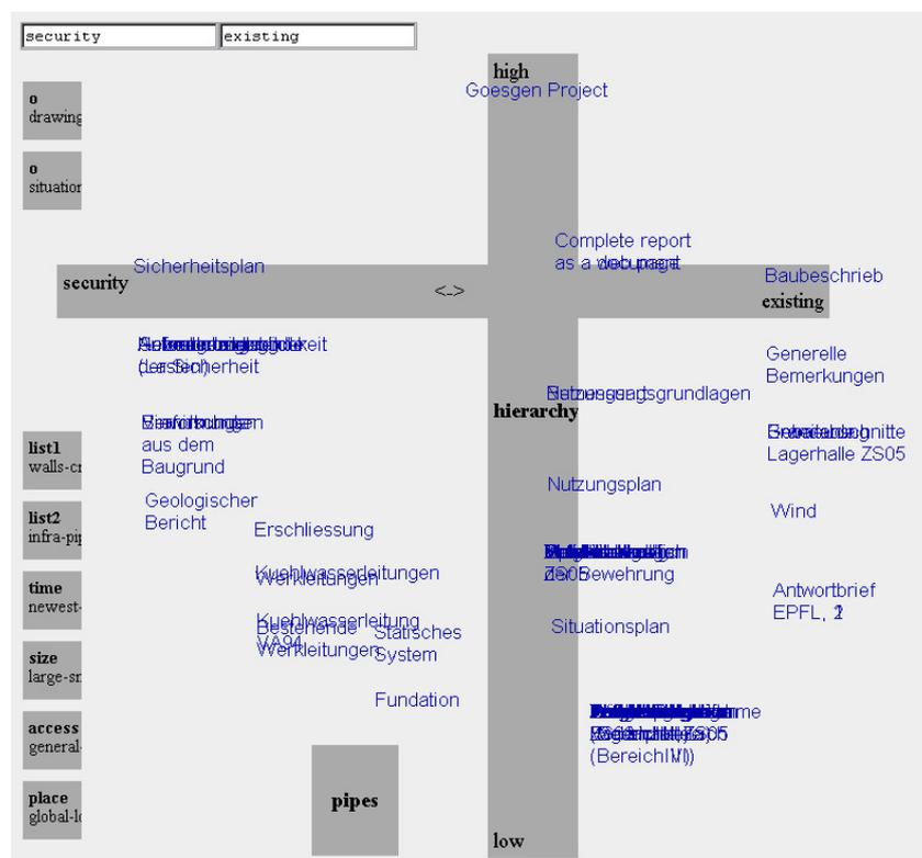
Figure 5. Snapshot of a dynamic visualization of a document hierarchy using attractors. Specifying a single category ('pipes') or a set of categories attracts documents that share one or more of these categories. Placing two categories in opposition ('security <-> existing') pulls documents to either end of the attractor corresponding to their categories. A third attractor is based on explicit grouping relations ('high hierarchy low'). David Kurmann.
