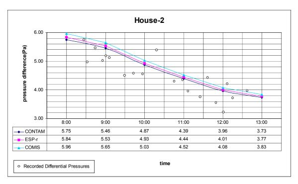
Figure 2 Measured and Predicted Differential Pressure across Garage-House Interface of House #2
