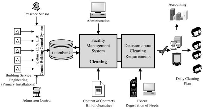
Figure 10. Registration and processing of the cleaning management
