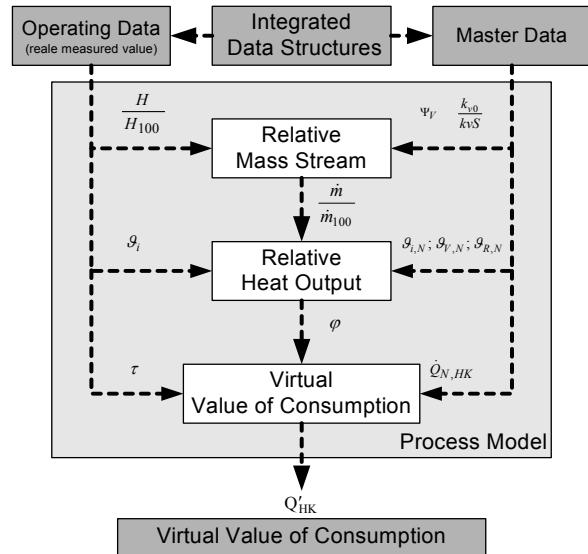
Figure 8. Process model of the virtual counting for a hot water heating with pumps
