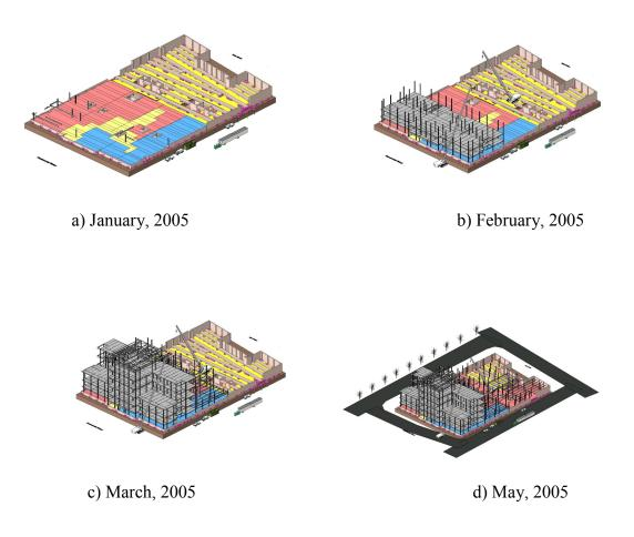
Figure 3: Gradual Progress of Steel Frame
