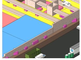
Figure 3: Object representing band beams, sub-grade, slab on grade and walls
