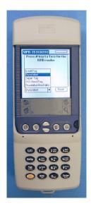
Figure 3 RFID Hand-held reader (www.rf-id.com)
