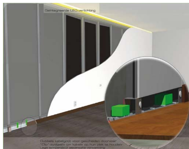
Figure 2: 3D- anisotropic section of the developed DCA-Wall
