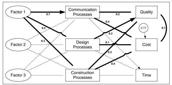
Figure 6: Example of a partial causality diagram of factors, processes and results. This diagram shows example values of the causality degrees only for the incidence between Factor 1 and Cost for clarity purposes.
