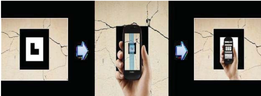
Figure 2: Tag detection leading to BIM model overlay and Snag information
