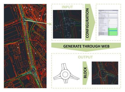
Figure 5: Generation of buildable drawings for a roundabout in the early phase of a project.
