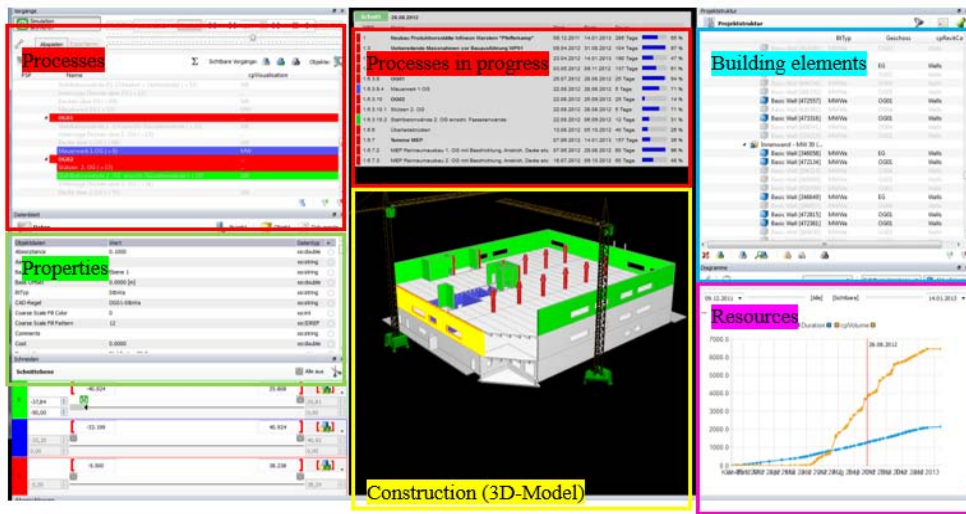
Figure 12. Construction control panel
