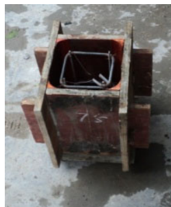
Figure 1. Mould with corner radius and reinforcement cage
