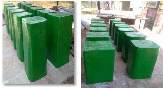
Figure 3. Views of GFRP wrapped prisms of different corner radii
