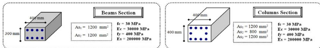
Figure 6. Beam, column cross sections and material properties.
