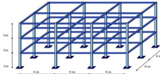
Figure 5. Geometry of 3D, 3-storey reinforced concrete frame structure.
