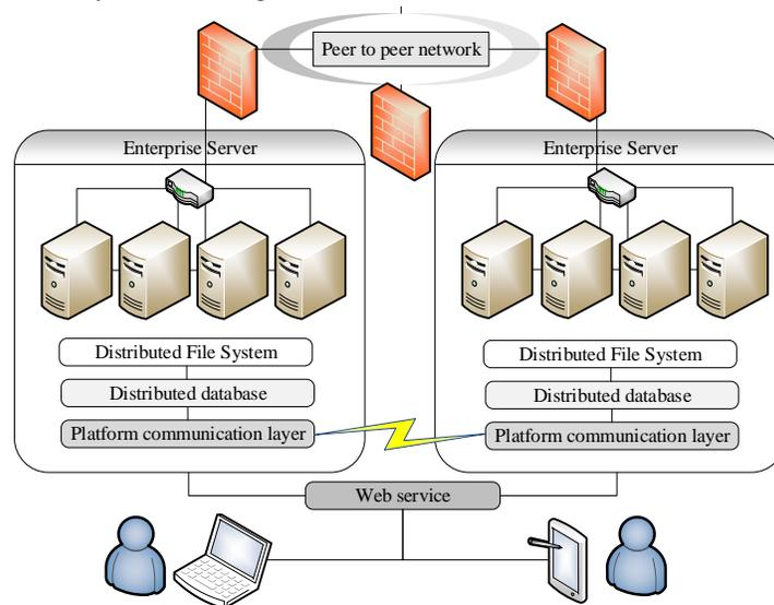
**Figure 3. The physical structure of distributed BIM service**
