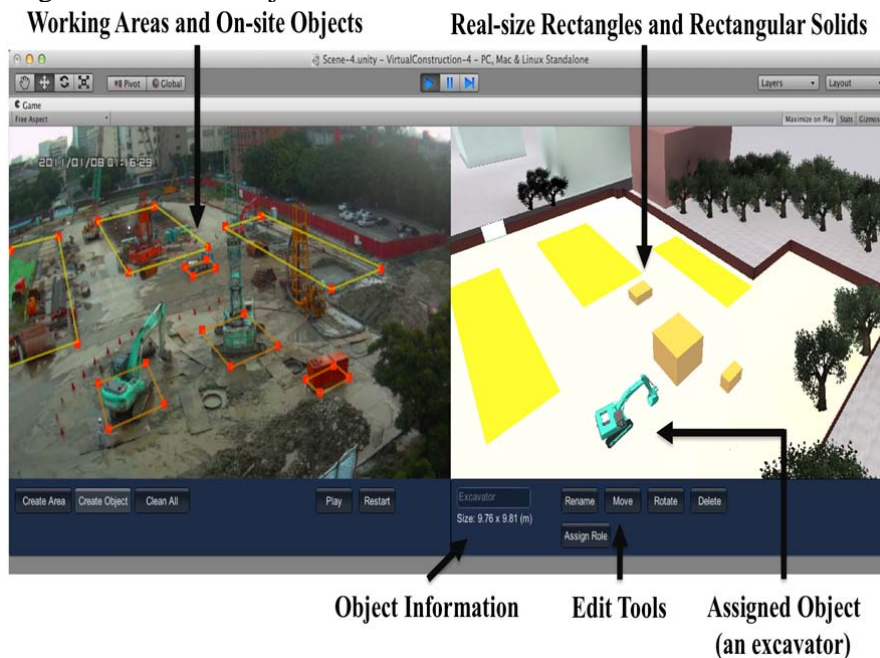
Figure 4. Planners can model working areas and on-site objects in the image as rectangles and rectangular solids in the virtual construction environment.
