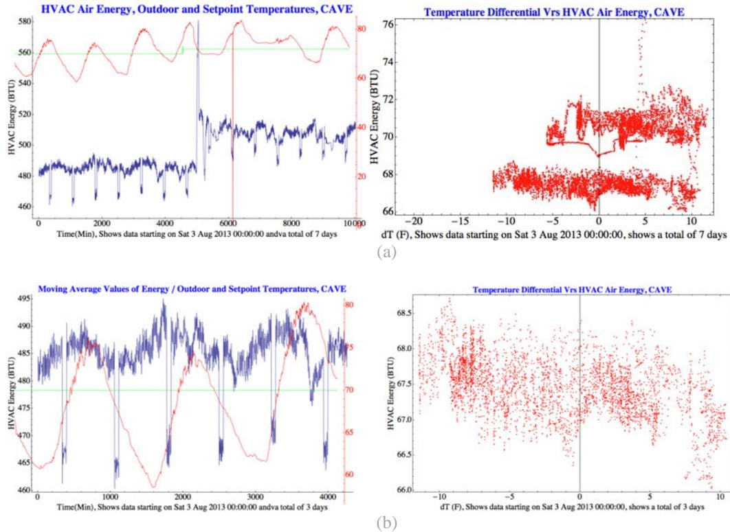
**Figure 4. Time Series and Scatter Plot to show an example of clustering due to changes in set point. (a) Shows period of 7 days with change in set point during 4<sup>th</sup> day; (b) Shows the first three days of period shown in (a)**
