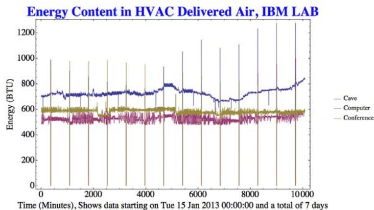
**Figure 2. Behavior of energy content in air delivered through HVAC system for the three rooms**
