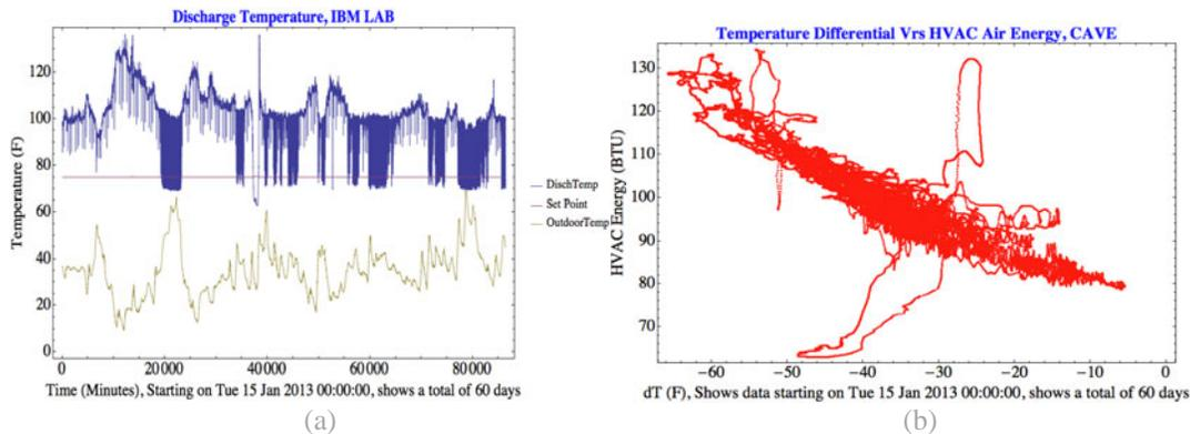
**Figure 3. Time Series and Scatter Plot to show an example of close relationship between exterior temperature and HVAC air energy content**
