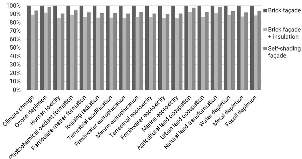
**Figure 4** Relative contribution of the three façade production and operation phases to the different environmental impact categories.
