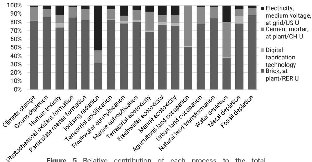
**Figure 5** Relative contribution of each process to the total environmental impact of the production of 1 m<sup>2</sup> of self-shading wall with the CH electricity generation mix.
