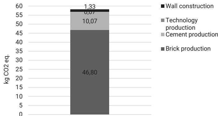
**Figure 7** Relative contribution of each process of self-shading system production to climate change impacts, considering 0% extra brick and CH electricity generation mix.
