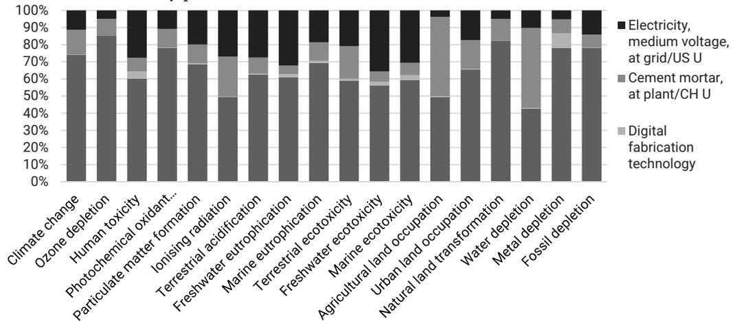
**Figure 2** Relative contribution of each process to the total environmental impact of the production of 1 m<sup>2</sup> of self-shading wall.
