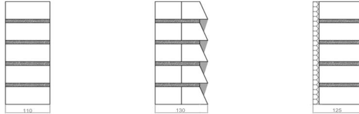
**Figure 1** Conventional brick, self-shading brick and conventional brick with insulation wall sections.
