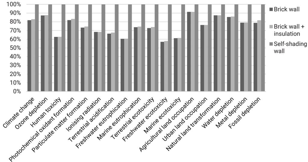
**Figure 3** Relative contribution of the three façade construction processes to the different environmental impact categories.
