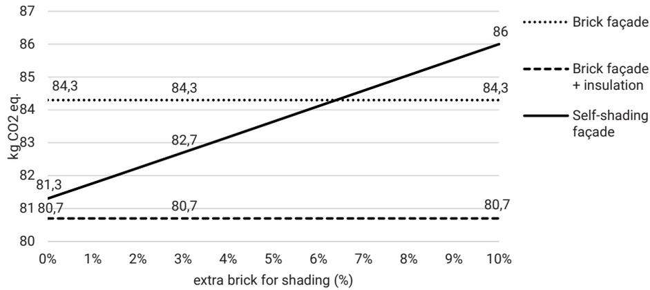
**Figure 6** Climate change impacts of the three façade systems during production and operation, in function of the extra brick considered for the self-shading façade.
