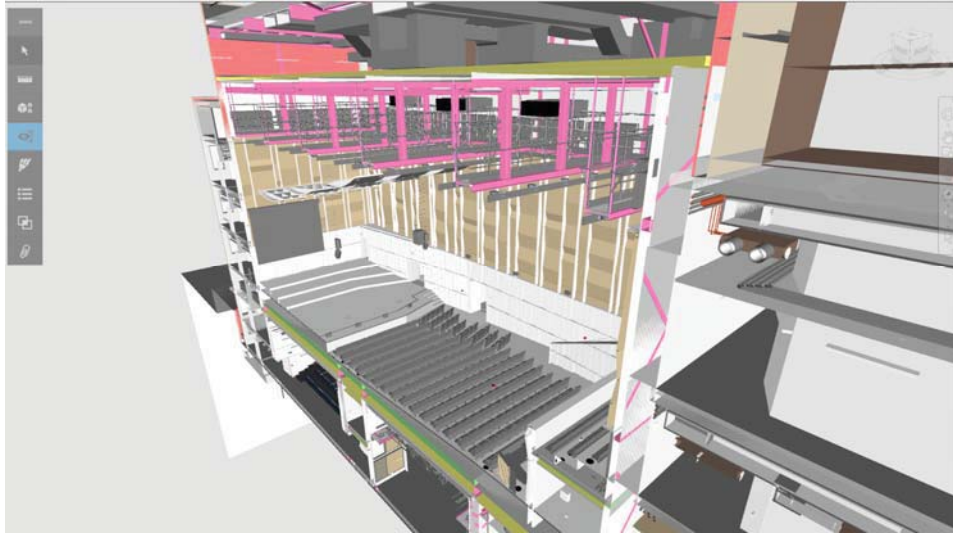
Figure 1. Federated model files used to find areas of 'clash' within proposed design scheme (Draper, 2015).
