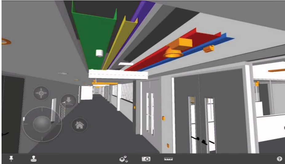
Figure 2. Model view of wiring cable trays captured and coordinated (as-built conditions) (Hall, 2015).
