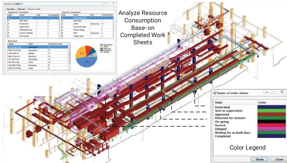
Figure 7 The colored 3D model reflecting order sheet's state and resource consumption statistics
