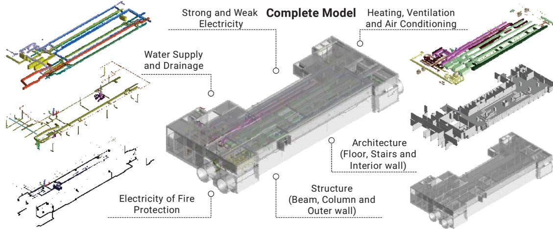
Figure 2 Integrate different models to establish a complete BIM model
