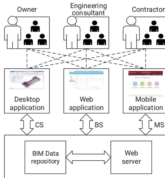
Figure 6 System logical components
