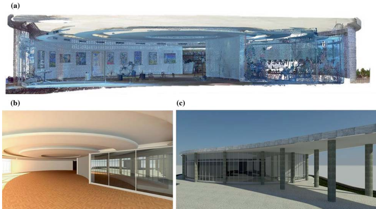
Fig. 4.5 Model of Ballroom: a point cloud section of interior; b rendered interior view of BIM model; c rendered exterior view of BIM model
