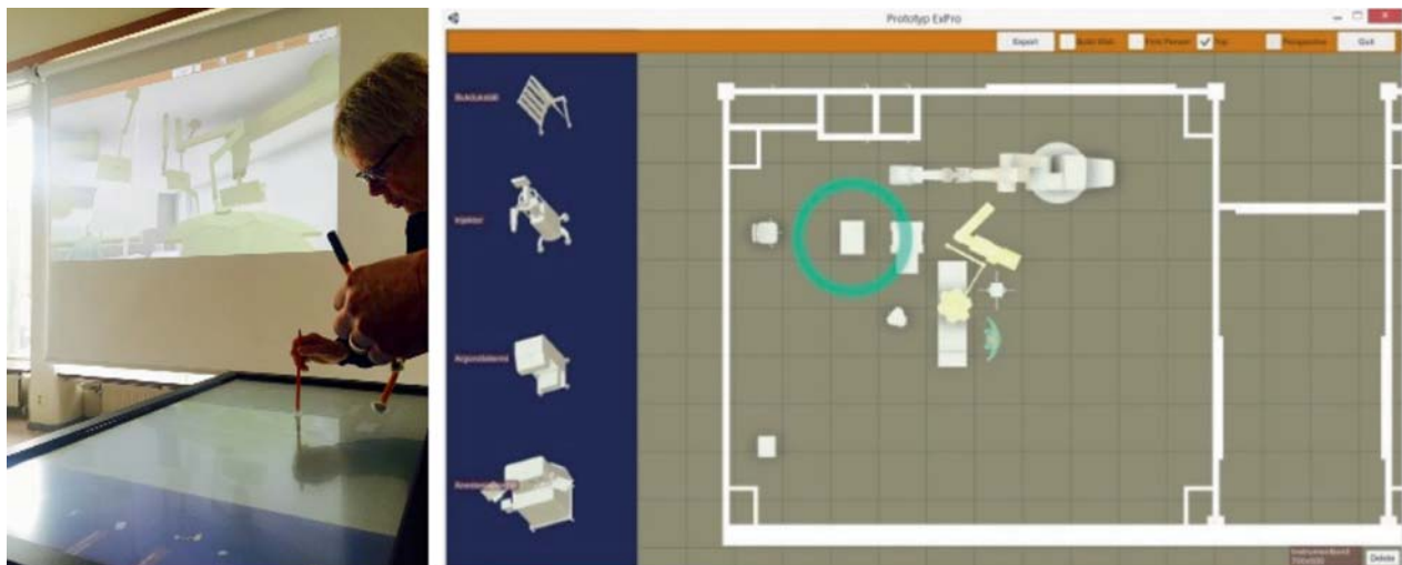
Fig. 32.2 Left: The multi-touch table used together with a non-immersive VR display, controlled by a wireless game controller (Picture from workshop 1). Right: The layout of the multi-touch table screen. Available components are accessible from a scrollable panel on the left side, and are added to the scene using drag-and-drop
