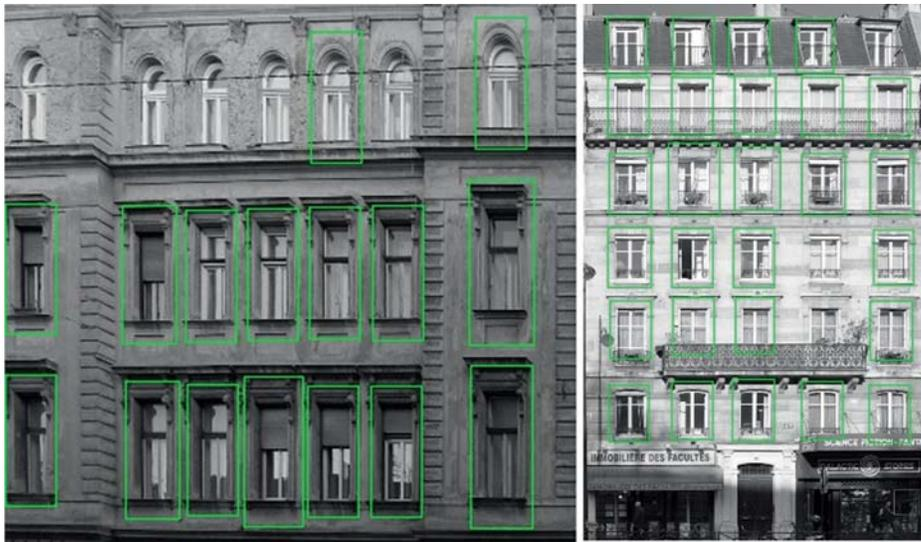
**Fig. 64.4** Window hypotheses obtained by our detector. Hypotheses are of different sizes and are slightly larger than the actual windows
