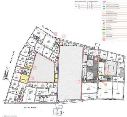
Figure 2: example of the fire prevention masterplan at the third floor of the building.
