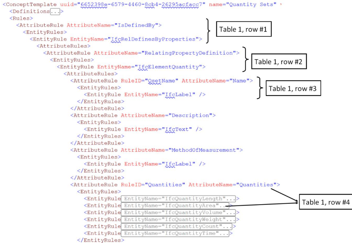
Figure 4: The XML format of the concept “Quantity Sets” and content mapping with Table 1
