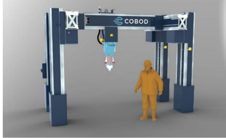
Figure 4. BOD2 3D printer (courtesy of COBOD International).
