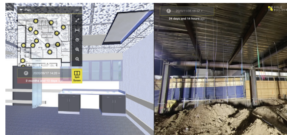
Figure 1: A HoloBuilder SplitScreen view displaying a 3D model scene and an active construction site scene
