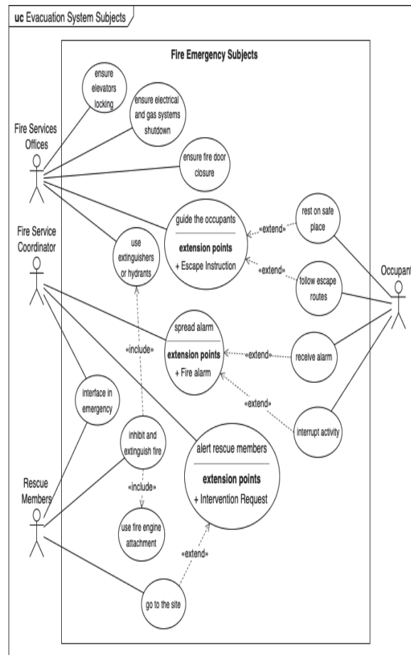
Figure 5 Evacuation Use Case Diagram (ES03)
