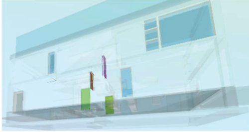
Figure 4: LD-BIM highlighting the four ‘non-compliant’ doors
