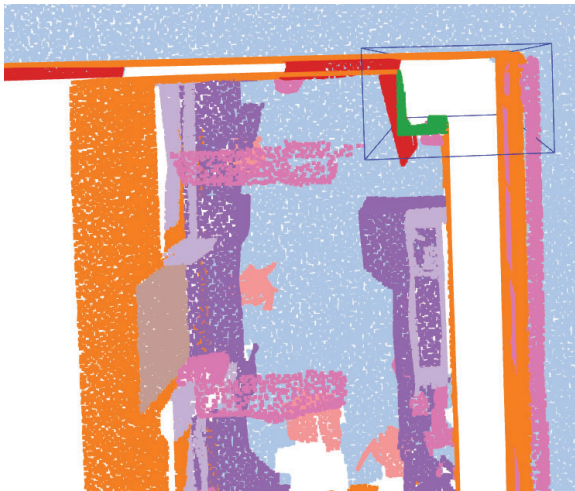
Figure 1 Ground truth cluster (dark green) and parametric model (blue bounding box) of a rectangular column.
