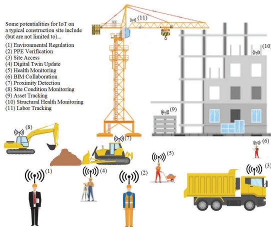
Figure 2: Typical Smart Construction Site Applications (Morman 2021)
