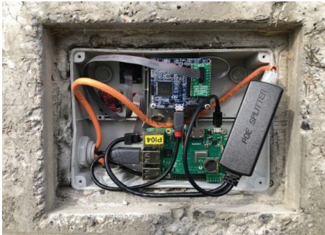
Figure 9: The prototype of SAB1 installed on the renovated bridge. SAB1 is equipped with a triaxial accelerometer and a biaxial inclinometer.
