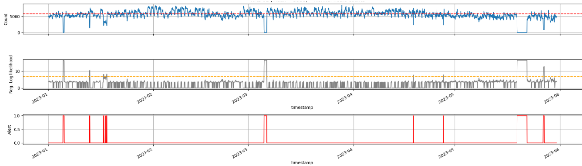
Figure 8. Anomaly detection with a Normally-distributed Streaming Data (NAE-01) Top: Count, Middle: Negative log-likelihood; Bottom: Alert Signal.
